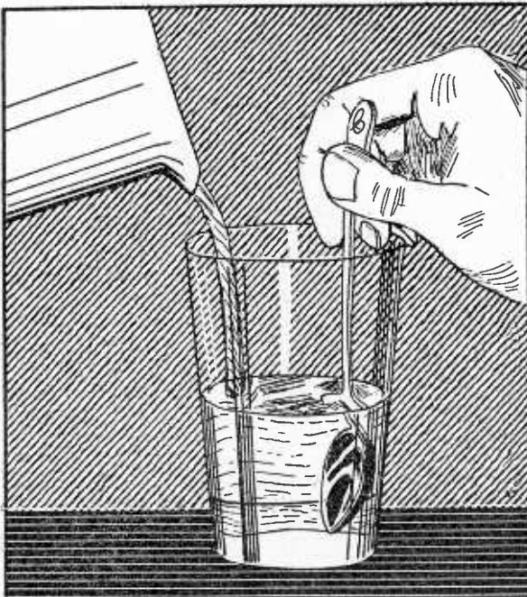
Fig. 1. Tea Glass Shows Principle of Cutting Down a Crystal to Adjust for Speed
